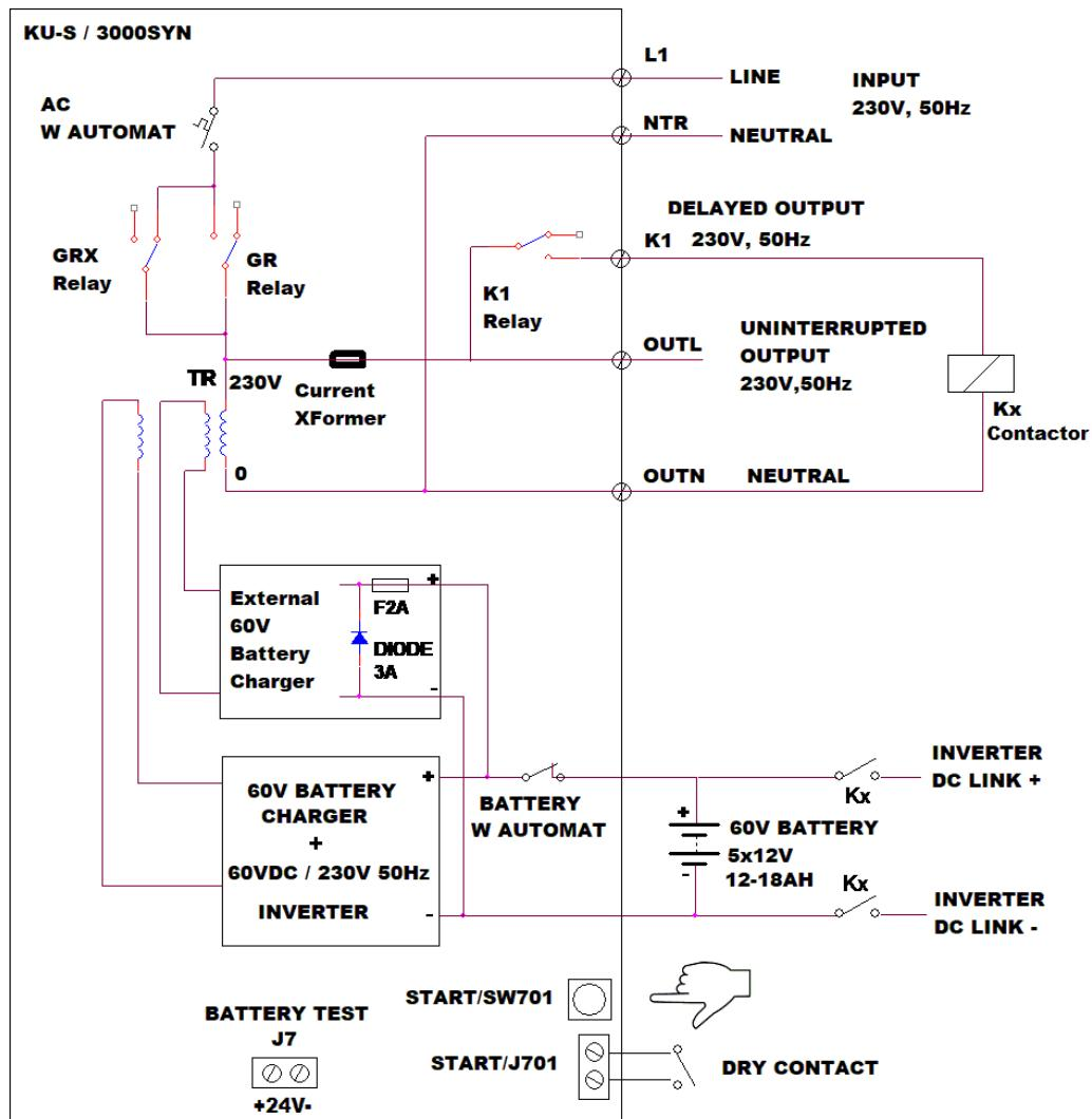
Note: The delayed output may be used to connect DC battery terminals to the inverter DC bara (bus) terminals, as shown above. Applying 24V DC to +24- (J7) Terminals gets the UPS into battery test mode while UPS is in main mode. To Start UPS manually(Cold Start Mode), press START(SW701) more than 2-3 seconds. To Start UPS remotely , there must be only **DRY CONTACT** connections at J701 terminals.
